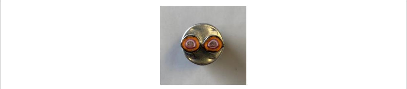
Figure 3.42: Representation 4.0 mm 2 SCC shielding sleeve fold (3.10.1 Cable shielding crimping using two half-shells)
