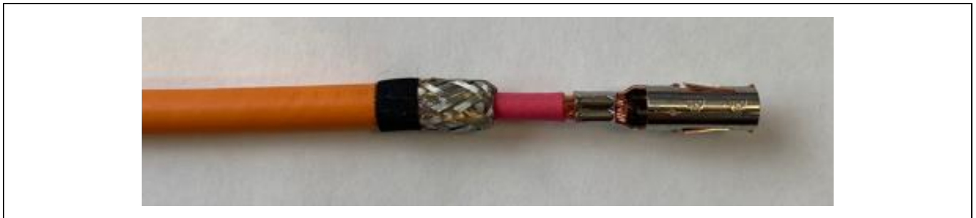
Figure 3.21: Representation 4.0 mm 2 SCC crimped HCT4 female terminal (3.6 Crimp the HCT4 female terminal)
