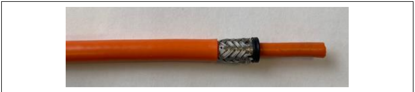
Figure 4.7: Representation 6.0 mm 2 SCC remove shielding foil (if present), trim shielding braid, and crimp the ferrule crimp (4.4 Remove shielding foil (if present), trim shielding braid, and assembly the stress relief and X-Ring)
