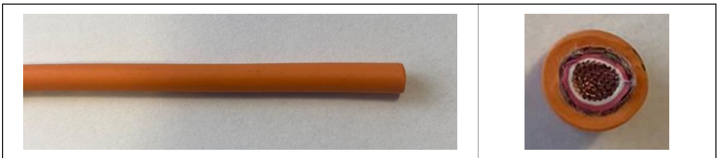
Figure 3.1: Representation 4.0 mm 2 SCC cable example (3.1 Cutting the cable)
