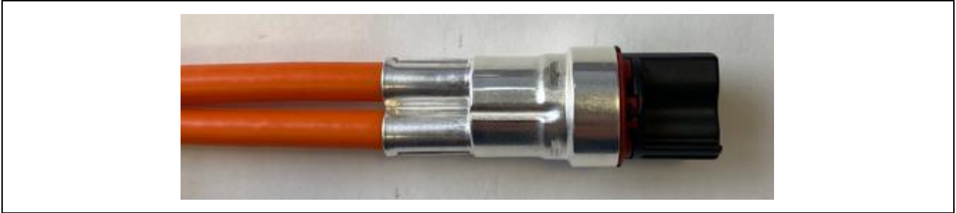
Figure 4.26: Representation 6.0 mm 2 SCC crimp the shielding sleeve (4.9 Crimp the shielding sleeve)
