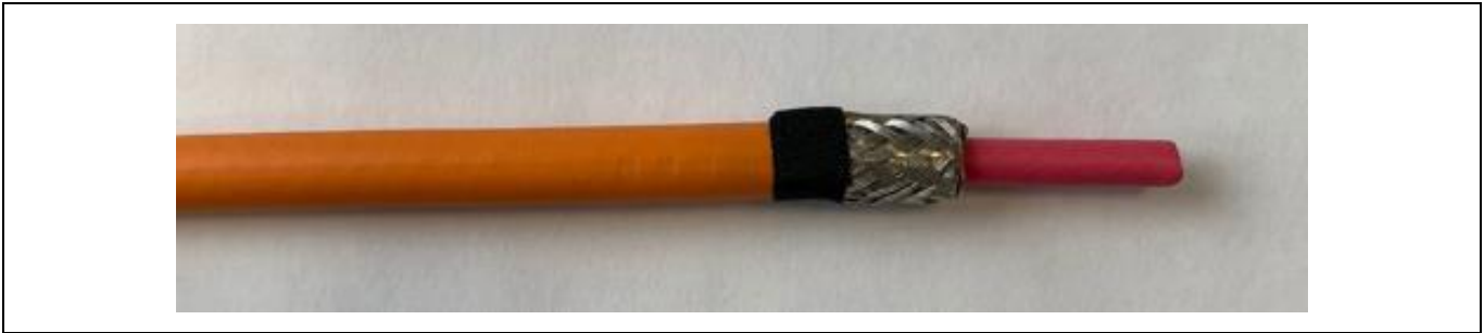
Figure 3.13: Representation 4.0 mm 2 SCC fold over the shielding braid and secure the shielding braid (3.5 Fold over the shielding braid and secure the shielding braid)
