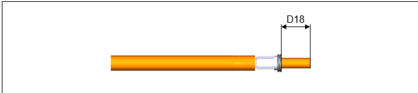
Figure 4.12: Representation 6.0 mm 2 SCC dimension D18 (4.4 Remove shielding foil (if present), trim shielding braid, and assemble the stress relief and X-Ring)
