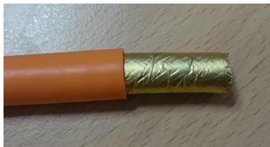
Figure 23: Strip off shielded cable
