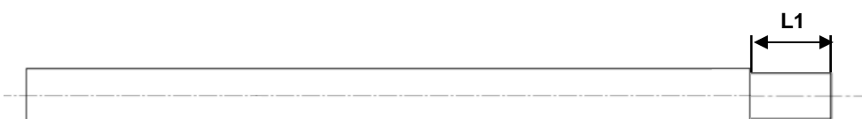
Figure 24: Stripping length L1
