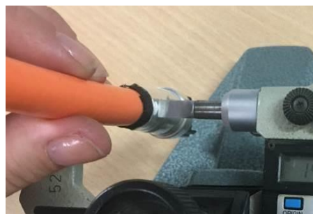
Figure 47: schematic representation of the measurement of the pressing height
