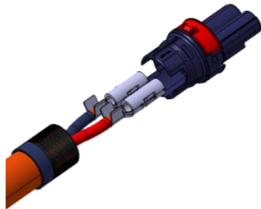
Figure 36: Assembly the female terminals into the contact holder
