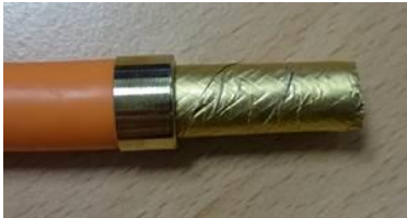
Figure 25: Assemble the stress relief
