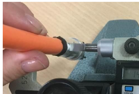
Figure 54: schematic representation of the measurement of the pressing height
