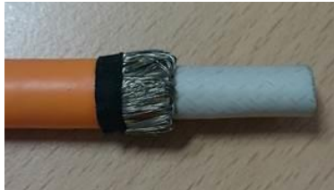
Figure 29: Fold over and fix the shielding
