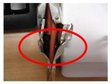
The wires on the inside of the distributor shall not be clamped.
